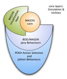
Figure 1: The basic BOD/MASON architecture. We have added extra layers of functionality on top of MASON's default layers (in keeping with MASON's design principles) which provide the user a simpler programming interface, including access to specialist action-selection code.
